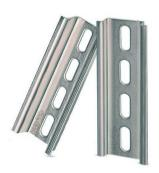
The TH35-7.5/s and TH-35-15/s rails are slotted products that are mainly used in electrical cabinets. The operator can use screws to fix the rail on the electrical cabinet. These products are made from cold roll steels and have an cold galvanized coating and a white chromate layer.
